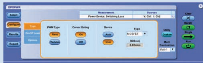
Figure 7. The DPOPWR input page allows the user to enter data sheet values for R_{DS_{ON}} & V_{CE_{sat}} .
