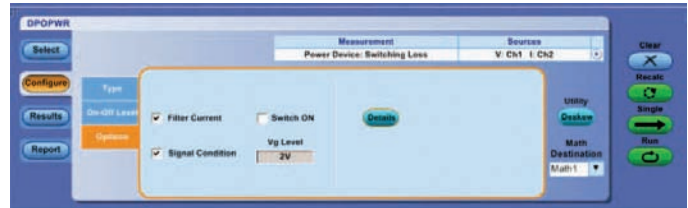
Figure 13. Signal conditioning option on the TDSPOWER3 software menu. This selection sets the current to zero during the “Off” time of the switching device.
