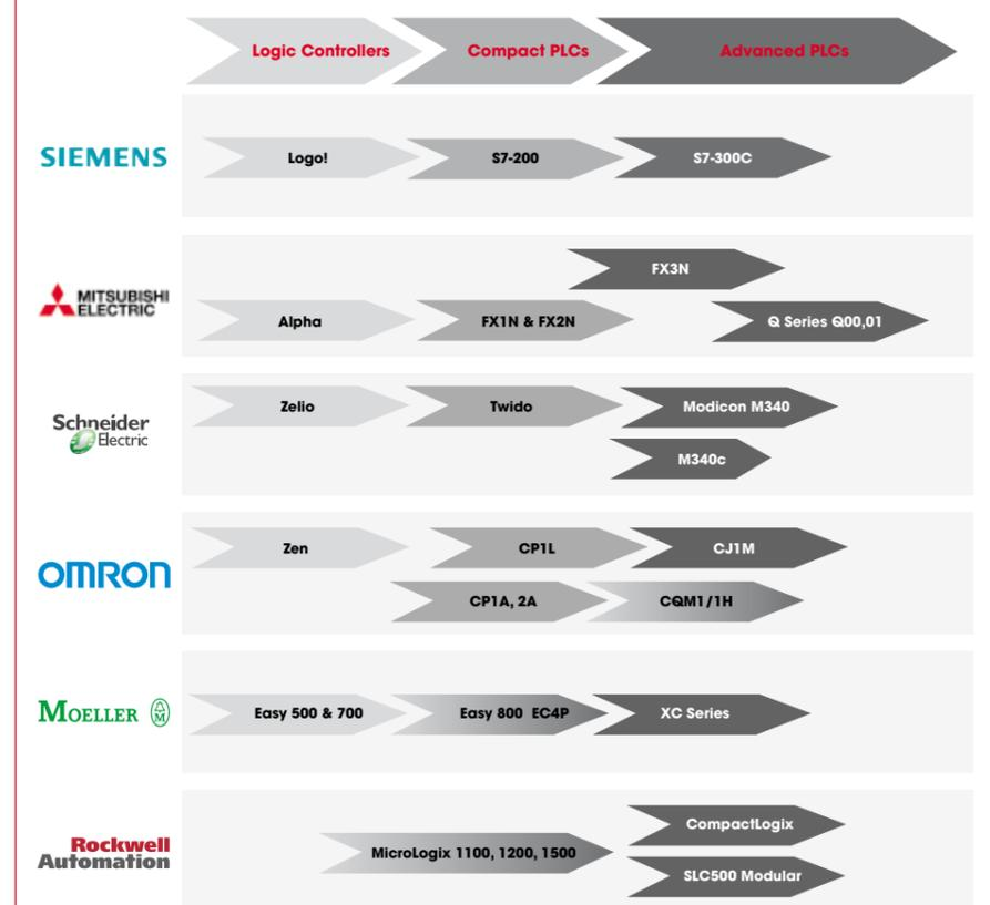
As a starting point you should only consider a logic controller for slower processes with an I/O requirement of less than 20 I/O. Beyond that level of I/O a compact or intermediate PLC provides a better solution with increased processing speed available. For large I/O applications with networking and remote I/O requirements an advanced PLC would be the best choice.
